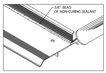
2. Miter & Scupper Anchor Bar (Preparation) Lay miters and spill out scuppers on deck with outside face down. Be sure aluminum anchor bar is clean and free of dirt or dust. Apply a heavy 3/8" bead of non-curing sealant to the right angle intersection of the deck flange and back of anchor bar as shown. Application of sealant is required along the full length of each miter anchor bar.
